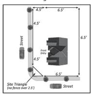
Fences exceeding 30 inches in height may not be placed within the 40 foot visibility triangle at intersections, or 10 foot visibility triangle where a driveway crosses a street, path or sidewalk. **See Figures 4, 5, and 6**.
