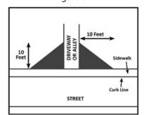
\*Regardless of Figures 4, 5, and 6, no portion of any fence shall extend into the city right-of-way. The right-of-way typically extends approximately 15 feet in from the edge of the curb. It is the property owner's responsibility to locate property lines prior to installing a fence.
